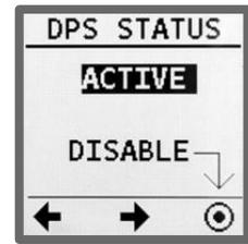
In cases where the DPS system is disabled due to error detection, **the DPS unit will activate an audible alarm**, and the remote, if available, will indicate the error on the screen. **The engines and thrusters will return to its neutral status immediately.**
